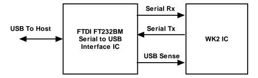
The block diagram above shows how the standard serial connection on the WK2 IC is fed to the FTDI chip which essentially converts it to USB format. The FTDI USB driver installed on the host PC presents the interface to Windows applications as a standard serial port so that the MSCOMM driver, or other serial driver, can be used.
