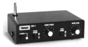
The ANC-4 is an rf device that eliminates or reduces power line noise, computer noise, TV-generated interference, and other types of electrical noise. The ANC-4 unit connects right to the antenna connector of the receiver or transceiver to cancel locally generated noise before it gets into the receiver and affects the receiver AGC circuits. Reception of signals well below the noise level of the local interference is possible.
